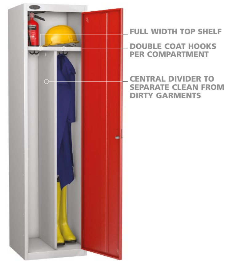
CLEAN & DIRTY LOCKER Complete with full width internal top shelf 305mm high, vertical centre partition and two double coat hooks. WIDTH 460mm DEPTH 460mm TOP COMPARTMENT HEIGHT 305mm
